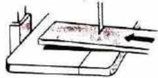
Fig 647 DO NOT LIFT UP THE BOARD THE SAW BLADE MIGHT BREAK
