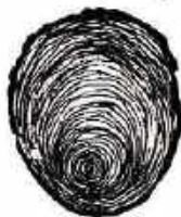
Fig. 17. TENSION WOOD ECCENTRIC PORTION OF STEM CROSS SECTION
