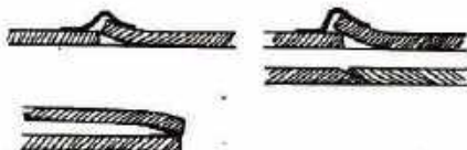
Fig. 84.(D) FAULTS WHICH ARISE WHEN THE GUM-TAPE IS EITHER TOO WET OR NOT SUFFICIENT PRESSURE IS APPLIED ON THE GUM-TAPE
