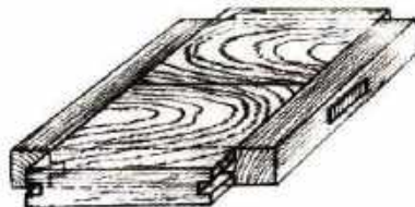
Fig. 60. PANELS WHERE TOO DRY
