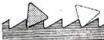
Fig.269(A) RIP-SAW (B) TEETH HAVE LESS THAN 90 DEGREES
