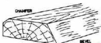
Fig. 656. A BOARD WITH A CHAMFER AND A BEVEL
