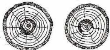
Fig.24. CUP SHAKE AND RING SHAKE
