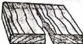
Fig. 59 CRACKED BOARD DUE TO RAPID DRYING
