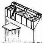
Fig. 511 MARKING THE PINS WITH A BEVEL PATTERN
