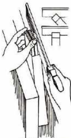
Fig 430 CUTTING A TENON WITH BACK
