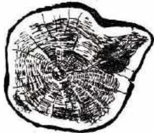
Fig. 21 FROST CRACK SHAKE
