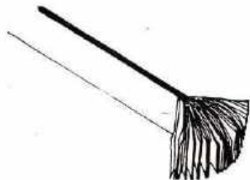
Fig.76 LAYERS OF COMPRESSED IMPREGNATED PAPER HAVING METAL-LIKE STRENGTH
