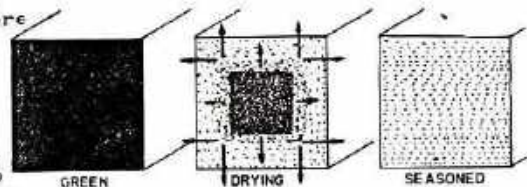
Fig 48. HOW WOOD LOSES MOISTURE
