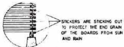
Fig.53 DETAIL OF STACKING LUMBER FOR AIR DRYING
