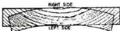
Fig.64 THIS SHRINKAGE AND WARPING ALWAYS OCCURS AGAINST THE ANNUAL RINGS. THE BOARD WARPS FROM RIGHT TO LEFT
