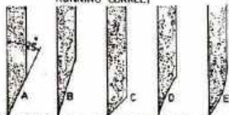
Fig.289. (A) BEVEL CORRECT (B) TOO LONG (C) TOO SHORT (D) TOO CONCAVE (E) TOO CONVEX
