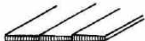
Fig.80. PANELS OF STRIPS WITH GROWTH RINGS AT RIGHT ANGLES TO FACE OF PANEL
