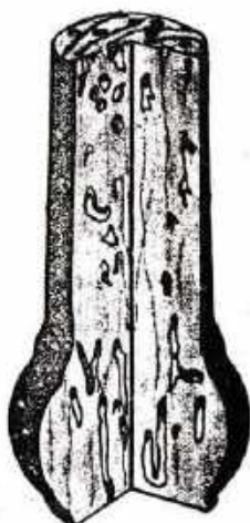
Fig. 31. LYCTUS POWDERPOST WORK IN HARDWOOD LUMBER VERTICAL SECTION
