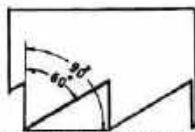
Fig.253 RIP AND CROSS CUT SAW TEETH
