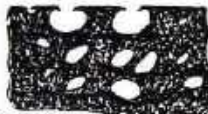
Fig.571. PORES CUT THROUGH AND FINE EDGES BENT DOWN BY PLANE OR SCRAPER
