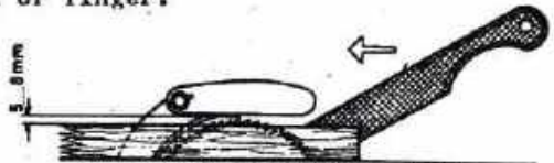
Fig.584. SETTING OF THE SAW FOR RIPPING
