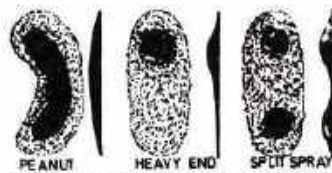
Fig. 580. CORRECT AND FAULTY SPRAY PATTERNS
