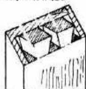
Fig. 516. MITER CHISELLED THEN PLANED
