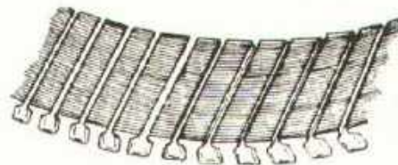
Cuffed insulation installed in slots
